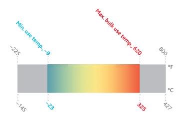
Eastman Therminol<sup>®</sup> 62 heat transfer fluid offers outstanding performance to 325°C (620°F), including excellent thermal stability and low vapor pressure. These properties result in reliable, consistent performance of heat transfer systems over long periods of time. The performance of Therminol heat transfer fluids has been proven through many years of industrial experience under a wide range of operating conditions.
